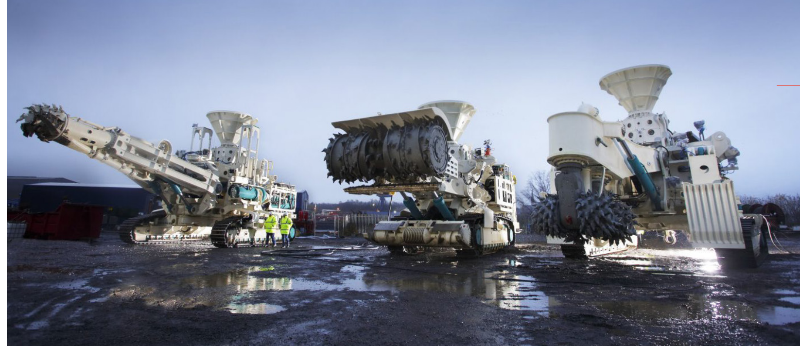
Image: Deep seabed mining machines manufactured by Nautilus Minerals (source: Nautilus Minerals)
